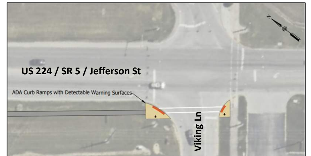
Plan view of proposed sidewalk and curb ramps at Viking Ln / Jefferson St intersection
