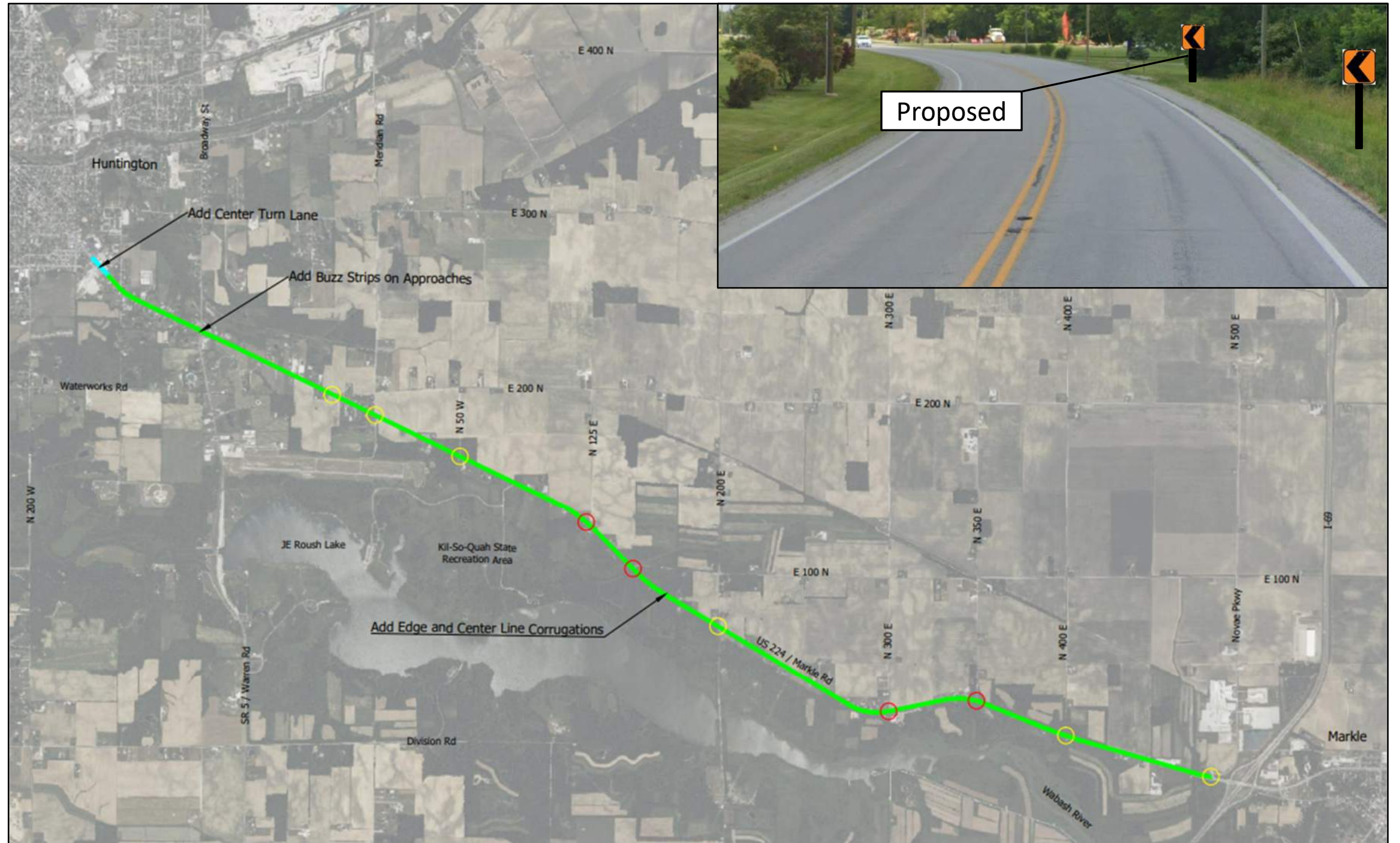
Summary map of US 224 corridor improvements. Example curve delineators on US 224 (inset)
