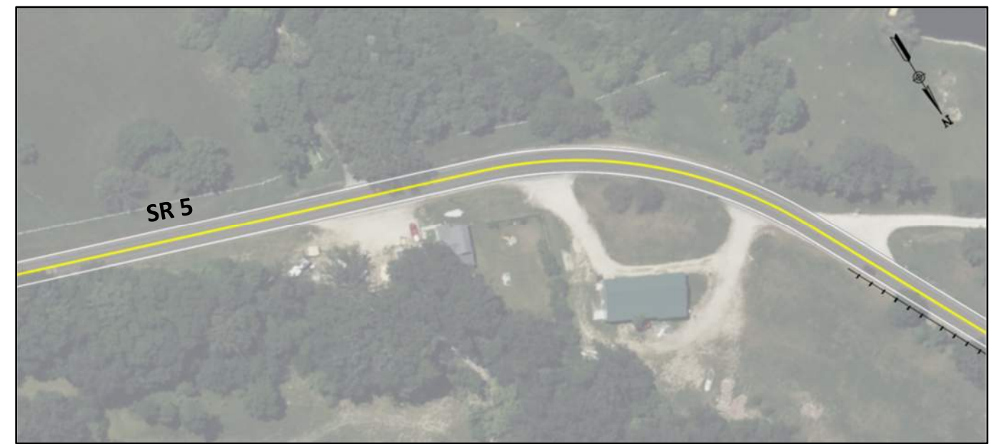
Plan view of proposed widening to curve west of Clear Creek. Road would be widened to include 12' travel lanes and 2' shoulders on each side
