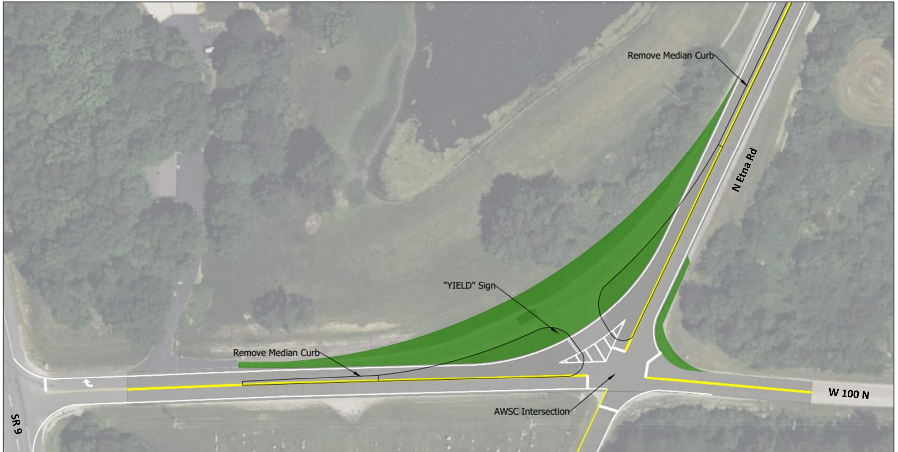
Plan view of proposed reconfiguration of Etna Rd / CR 100 N intersection to a conventional All Way Stop Controlled intersection.
