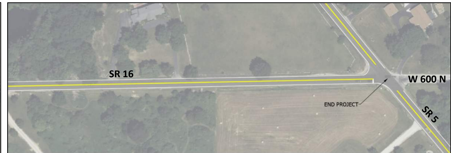
Plan view of eastern limits of SR 16 widening at SR 5 (SR 5 widening shown)
