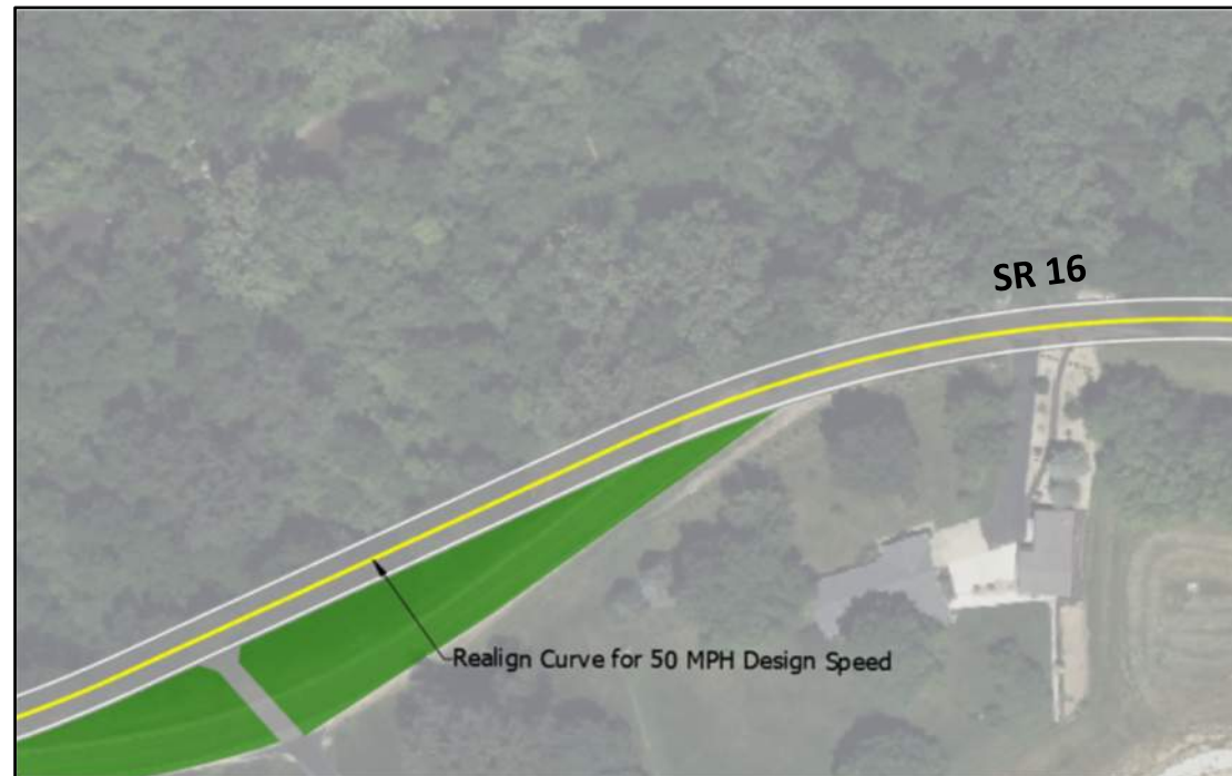
Plan view of proposed widening and curve realignment of SR 16 to include 11' travel lanes and 2' shoulders
