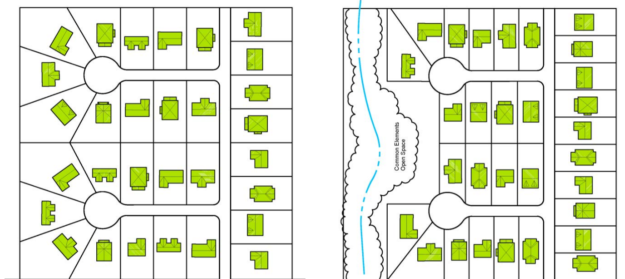
Figure 2-3: Traditional vs. cluster development. Both plans have the same total acreage and number of lots, but cluster development allows for smaller lot sizes and more common open space. Source: City of Greensboro, NC Land Development Ordinance, §30-7-3-3.3 (via enCodePlus.com).
